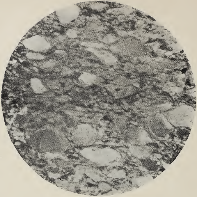
Fig. 1. Schistose Sandstone, Queen Bee Mine. Crossed Nicols, 1 inch mag.
